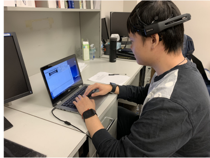
Fig. 1. Experimental setup. A user is typing on his laptop, and the brainwave signals are being captured using a 14-channel Emotiv Epoc+ headset. The hand movements are being captured using Sony smartwatch motion sensors that the user wore on his wrist. Data collection experiments were conducted in two separate phases. Although the figure shows EEG data recording using the Emotiv Epoc+ headset, phase I data collection experiments were conducted using a NeuroSky headset, whereas EEG data in phase II was collected using an Emotiv Epoc+ headset. In addition, hand movements from one hand of the user were recorded in phase I experiments, whereas movements of both hands were captured in phase II experiments.
